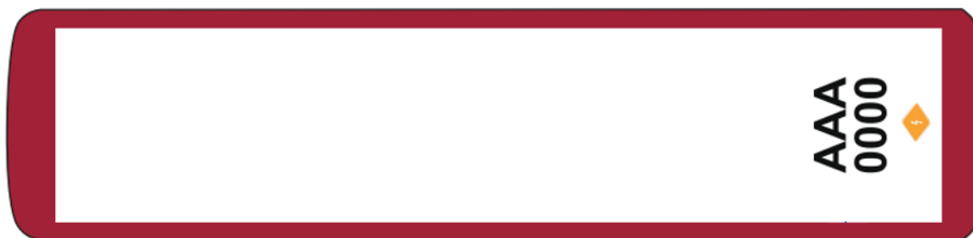
Figure 10_5 Roof Propulsion Identification Symbol location
